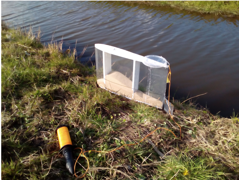
Figure 18: The model ship before the trials. Fixed-rudder to port, retrieving-line (orange) attached, ballast filled and trimmed.
