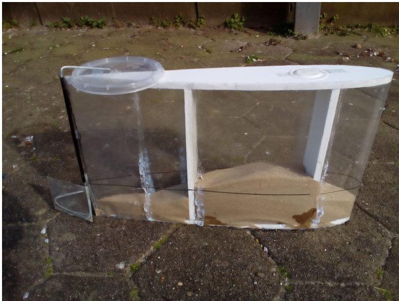
Figure 19: The disintegrating model ship after the trials. The glue dissolves, the hull shows leaks.
